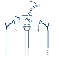
**3.** Remove the lid by turning it to a 30 degree angle and moving it downwards by introducing the side of the lid without the pressure relief valve.
