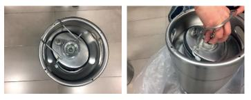
2. Introduce the lid completely and align it with the oval neck.
